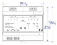
The DIN-I08 is a DIN Rail-mounted automation control module that provides eight Versiport I/O ports for interfacing with a wide range of third-party devices and systems. Each Versiport can be configured via software to function as a digital or analog sensing input or as a digital trigger output.
